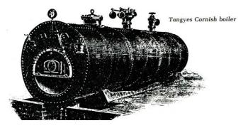
There was a great deal of equipment on site including immense Cornish boilers, seen above, weighing 22 tons for raising steam by the waste heat from the furnaces. There was a 1½-ton steam hammer, massive shears for cutting up double-head 75lb per yard rails into lengths, a large gantry, a 36in horizontal condensing 175-horse power engine and giant flywheels with a 30ft diameter and weighing 40 tons.
