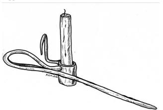
Some of the early candle holders were simply just a spike and miners used cotton thread, cloth tape or wire to attach a tallow candle. Later top hooks, 'handle' and candle holder, sometimes a thumb lever to push up the candle or push out the last bit of candle, these types being made by a blacksmith. The Americans often referred to these mining 'tools' as a 'Tommy Stick' or 'Sticking Tommy' to hold a candle though they had some that could hold a lamp as well.
