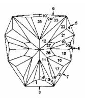
Angles for R.I.  $\Rightarrow$  1.760 62 + 9 girdles = 71 facets 1-fold, mirror-image symmetry 96 index L/W = 1.035 T/W = 0.575 U/W = 0.446 P/W = 0.473 C/W = 0.188 Vol./W<sup>s</sup> = 0.270
