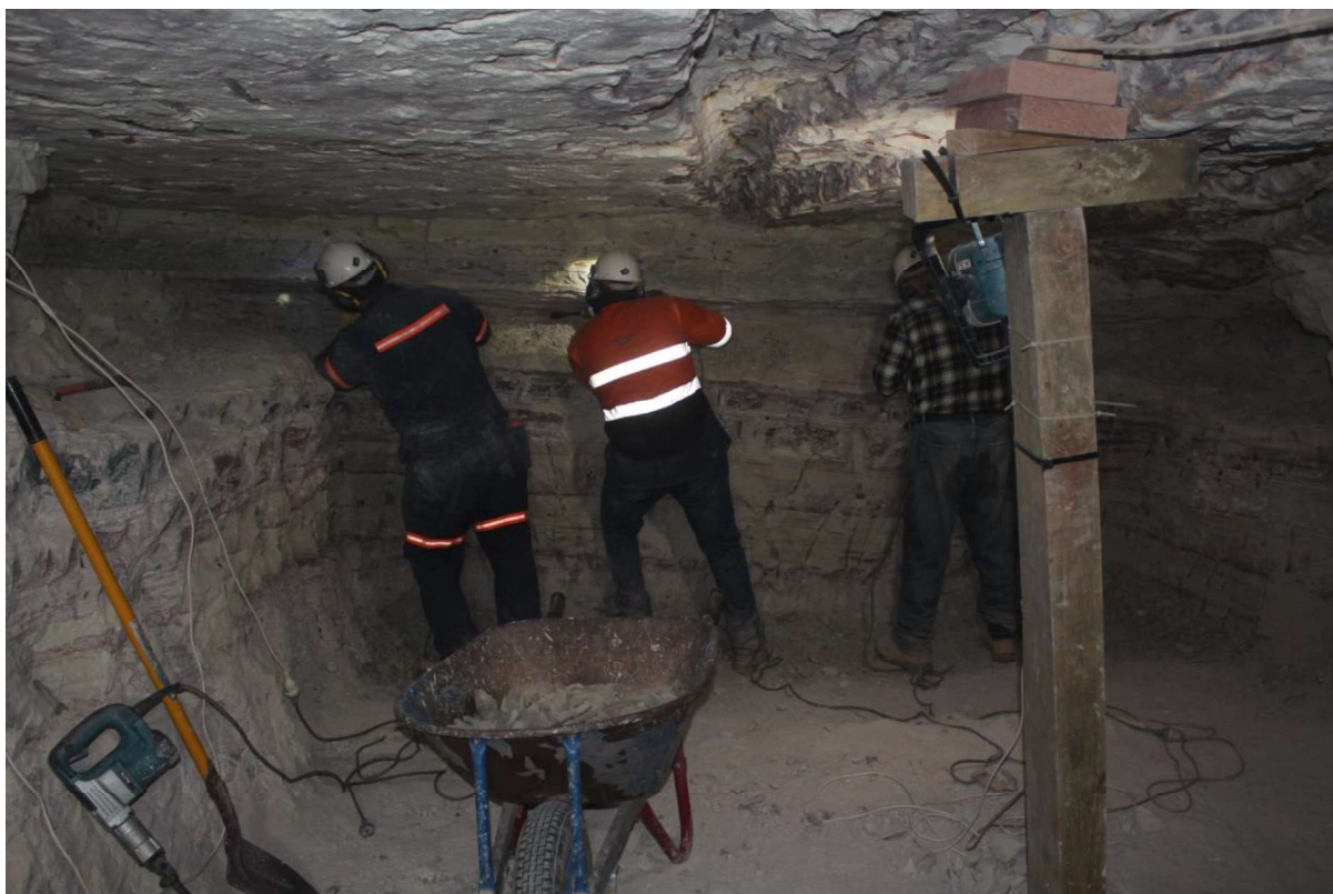
Photo 3. The USA family team in harmony preparing a half metre deep undercut using 900 watt Makita hammer drills with wide blade cutting tools sharpened by the local butcher in Alice Springs and kept in running order by the Pope family in Hobart. Left to right is Steve Scott, Daniel Scott and Bob Callum. Adit face photo.
